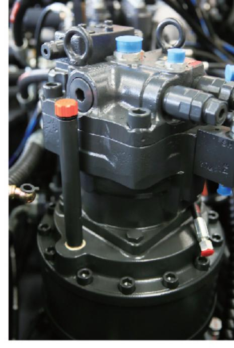
High-efficiency large-displacement motor, the rotary motor increases the displacement and increases the rotary torque of the whole machine by 12.1%
